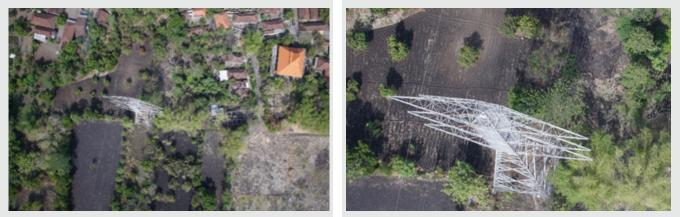
*Indonesia.* Camera Sony a6000, flight altitude 220 m above ground and 180 m above tower. Overall image quality is good but due to high flight altitude wires are overlapping and are slightly blurred.
