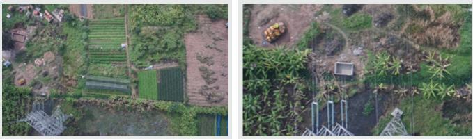
*Indonesia Udara*. Camera Sony a6000, flight altitude 150 m above ground and 110 m above tower. Images are slightly blurred, wires are overlapping themselves and dark.
